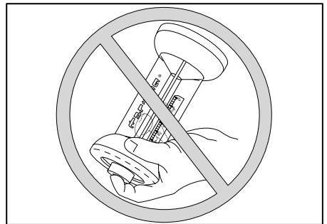
Figure 1d. NEVER vent FYRITE in the inverted position, which will cause fluid to spill.
