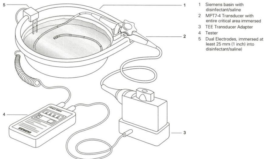
Example of Leakage Current Tester Setup for the SONOLINE G60 S system's MPT7-4 TEE Transducer.
