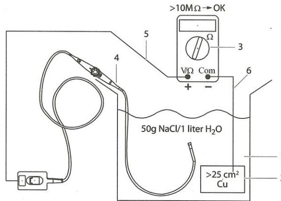
Figure 2 Equipment Used to Detect Bite-Holes in the Endoscope Shaft
