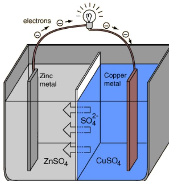
**Example of a Simple Voltaic Cell**
