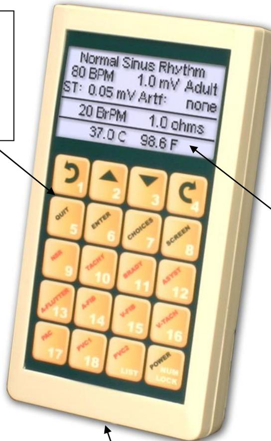
LCD Graphical Display with Backlight:
