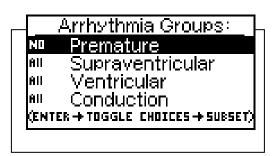
4. To select some of the arrhythmias in a group, use to display the list of arrhythmias for a specific group. Then use to scroll through the arrhythmias. Any arrhythmia marked with a check ( ,, ) will be included in the subset. Use to toggle the selection of an arrhythmia on and off.
