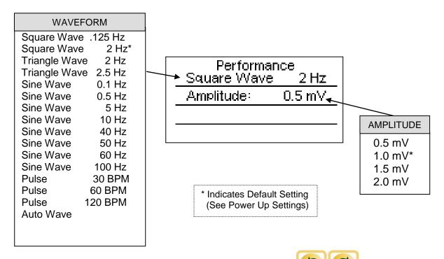
These waves and amplitudes can be selected by using to highlight the parameter to change and using to scroll to the desired option. Then is used to accept the new setting.
