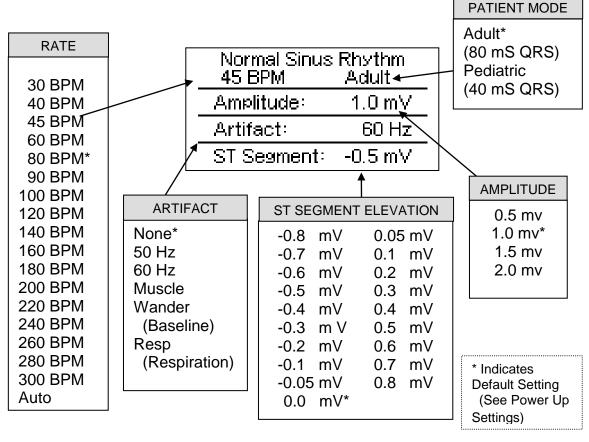
The rate, amplitude, adult/pediatric, artifact and ST elevation or depression can be selected by using to highlight the parameter to change and using to scroll to the desired value. Then is used to accept the new setting.
