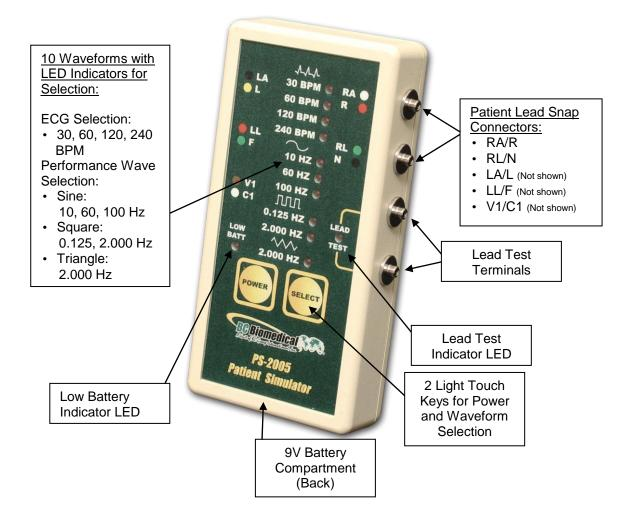
The unit is controlled by 2 light touch keys. They allow the user to select waveforms and control the power for the unit.
