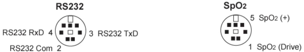
**NOTE: Mini-DIN pinout viewed from NIBP Connector Side**
