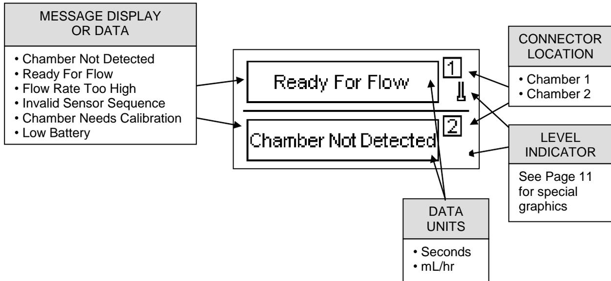
**CONNECTORS SCREEN** – The connectors screen indicates the layout of the connectors at the top of the IPA-1000. Also shown is the volume capacity of any connected Chambers.
