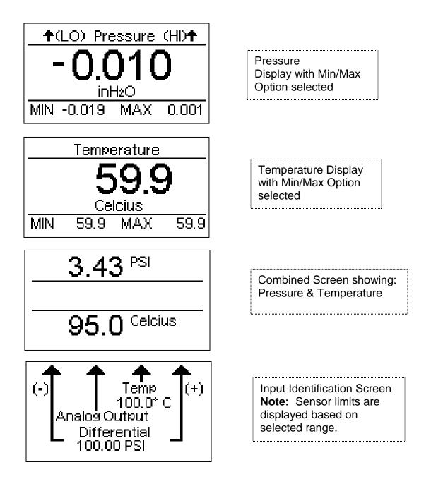
PRESSURE SCALE - The pressure scale is indicated by the units displayed under the
