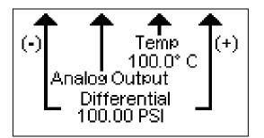
Input Identification Screen **Note:** Sensor limits are displayed based on selected range.
