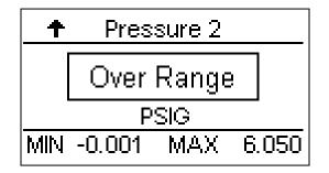
Typical display with "Over Range" message box. TEMPERATURE SCALE - The temperature scale is indicated by the units displayed under
