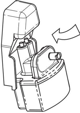
The unit has a front-mounted water trap. The trap slides out and can quickly be replaced if it becomes occluded. Use the designated water trap for this device (BC20-43001). The water trap has a fitting located at the top that connects into the trap receptacle (gas manifold) of the analyzer. The unit's gas sampling connection (from the water trap) accepts gas sampling lines using the male Luer style connections.
