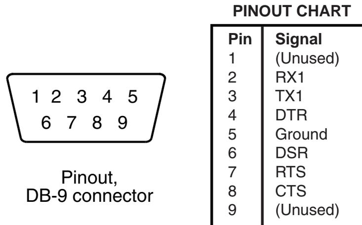
**Figure 7-1: COM1 Pinout Diagram**
