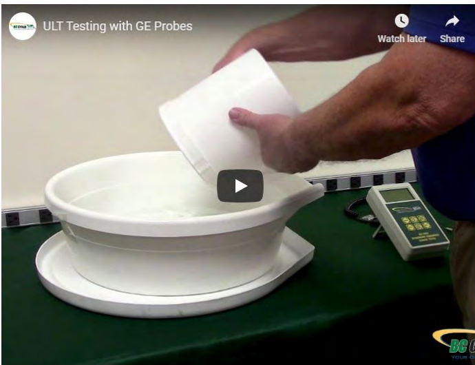
How to Perform an Ultrasound Leakage Test on GE Probes 6VT-D, 6Tc and 6Tc-RS
